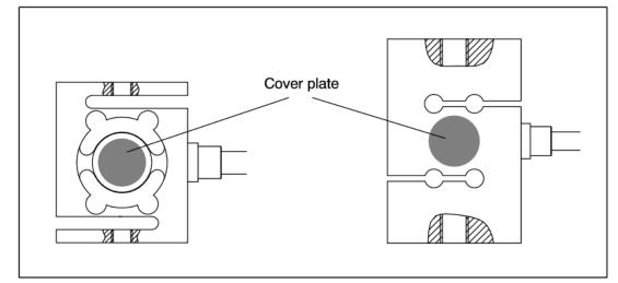
Load cell orientation during installation - load cell range from 10N to 1000N:
