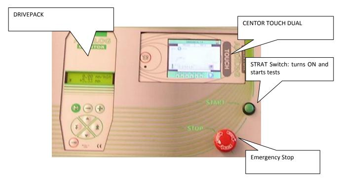
By switching ON the button on the side of the test stand and if the emergency button is not in down position, the DRIVEPACK will not turn ON. To start the CENTOR TOUCH, push its ON/OFF button: a general screen appears for 5secondes and then the main measure screen is displayed.
