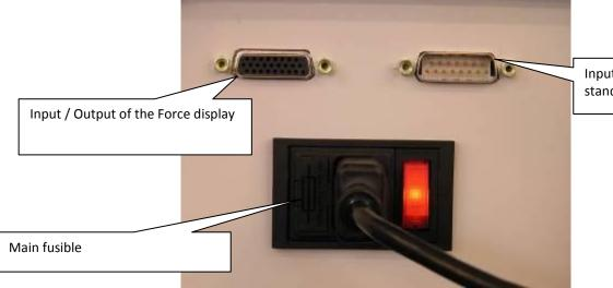
Input / Output on the motorized stand.
