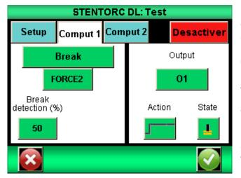
From the "Test" menu, "comput 1" tab, choose "break" from the available calculation and FORCE2. Set the percentage of the breaking force to 50% by example.
