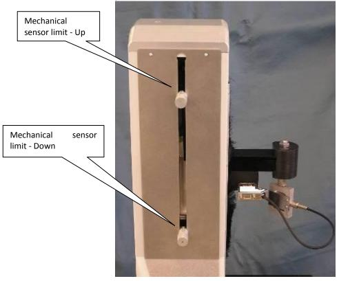
You can configure activation of your mechanical limits on the Drivepack menu at "Senor stop  $\mathbf{T}$ " and "sensor stop  $\mathbf{L}$ ".
