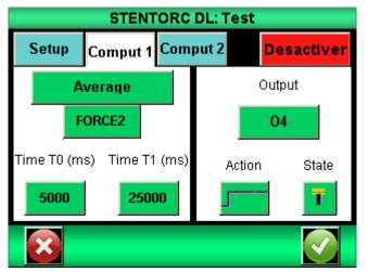
In the menu "test", press tab « Comput 1 », then choose Average and FORCE2. Setup Instant T0 to 5000ms and Instant T1 on 25000ms. Then validate
